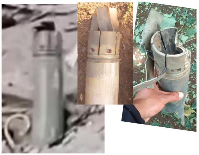
Figure 11: Visual comparison of remnants from Shiloh Baptist Church to confirmed S-8-type rockets' fins sections. (Sources: Private; <u>Guns.allzip</u>; <u>KNU</u>).
